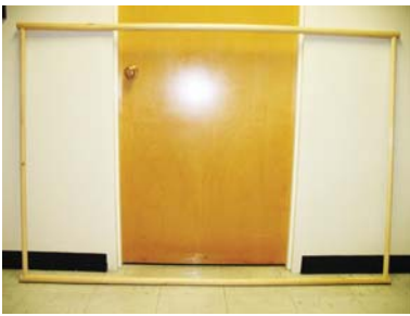
1. Make a frame about 72" long by 48" high. Use wood or PVC pipe and elbow joints.
