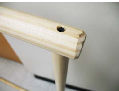
2. Drill a hole in the top and bottom pieces and attach the sides with screws.
