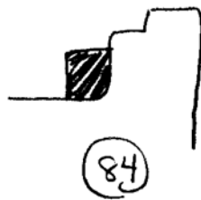
Figure 2.74. Room C-13, profile of bench at east end of south wall. This sketch indicates the two stage construction history of the bench.
