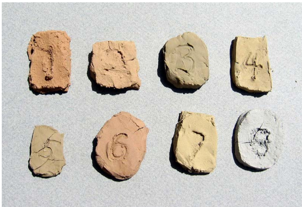
Figure 10. Numbered clay samples (briquettes) before firing.
