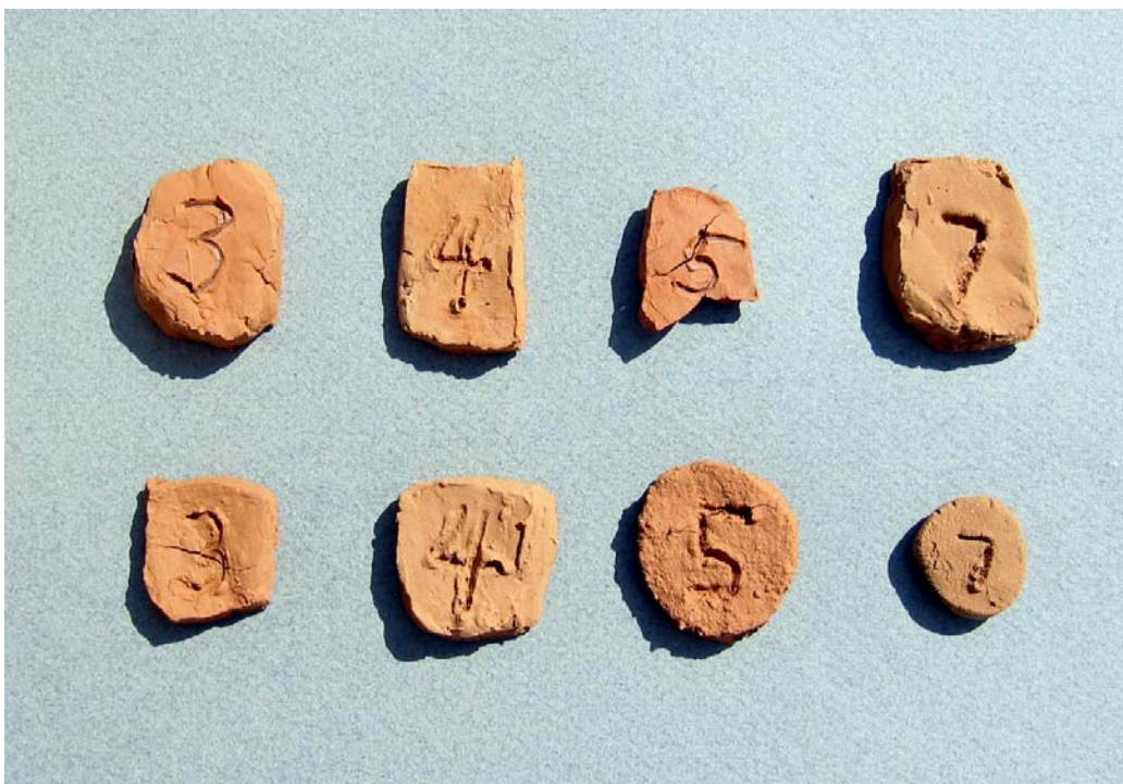
Figure 12. Numbered clay samples (briquettes) after second firing to 750 degrees C. The lower-fired samples are in the lower row, while the samples fired to 900 degrees C are in the upper row.
