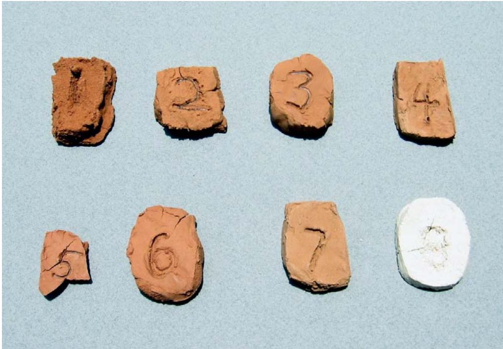
Figure 11. Numbered clay samples (briquettes) after firing to 900 degrees C.
