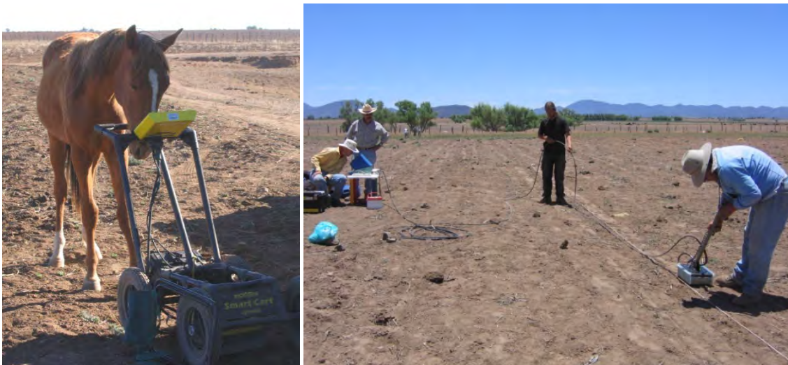
Figure 42. GPR survey devices. Left: Calgary device. Right: INAH device.
