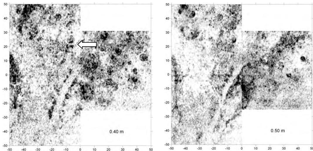
**Figure 10.** Alderete site: anomalies at depths of 40 and 50 cm. The two anomalies chosen for testing are indicated by an arrow on the left image.
