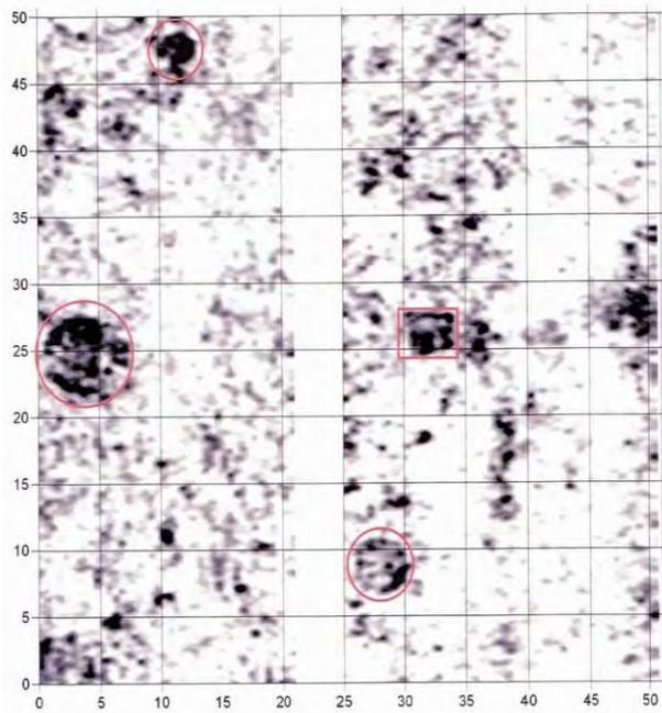
**Figure 28.** Ch-240, GPR scan at a depth of 40 cm. This image also shows the possible community house and one of the two smaller houses seem at 25 cm. A rectangular anomaly is also present.
